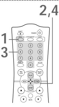
Press the PLAY/▲ button or the STOP/▼ button to select SMARTLOCK. Then, press the F.FWD/► button.
